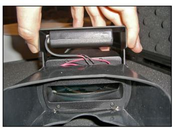
**VERY IMPORTANT – To Open & To Close** – Apply Pressure to the End of the Battery Cover to Release the Catch and Slide The Cover
